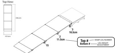
\* Stage not included with ramp \*Guard Rails Not Shown in diagram
