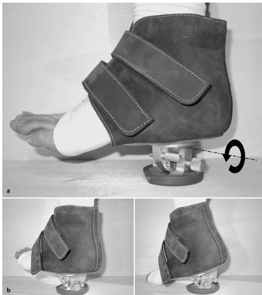
Fig. 1 a and b a Lateral view of the device used in the study, the dotted line represents the destabilization axis. b Illustration of the subtalar joint destabilization induced by the device. When the subject steps (left), the shoe rotates around destabilization axis, eliciting an inversion and plantarflexion movement of the ankle (right).
